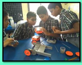
Students assembling Swift base robot. Swift base robots have 4 wheels, 4 drive motors and use skid steering.
